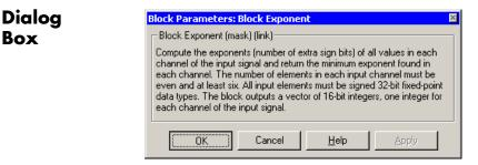
Algorithm In simulation, the Block Exponent block is equivalent to the TMS320C62x DSP Library assembly code function DSP bexp. During code generation, this block calls the DSP bexp routine given to produce optimized code.
