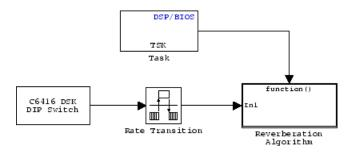
Normally, the algorithms in this type of task run in free-running mode, that is, they run repetitively and indefinitely. However, in this function-call subsystem (shown in detail in the following figure), ADC and DAC blocks suspend the execution of the task until the ADC and DAC data is available.
