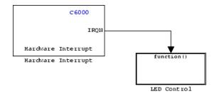
In this model, the C6000 Hardware Interrupt block installs a task that runs when it detects an external interrupt. This task then toggles an external C6416DSK LED on or off.
