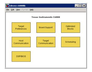
If you do not see the listed libraries, or MATLAB software does not recognize the command, install the target support package. Without the software, you cannot use Simulink and Real-Time Workshop software to develop applications targeted to the TI boards.
