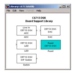
The C6713 DSK ADC and C6713 DSK DAC blocks generate code that configures the codec on your C6713 DSK to accept input signals from the input connectors on the board, and send the model output to the output connector on the board. Essentially, the C6713 DSK ADC and C6713 DSK DAC blocks add driver software that controls the behavior of the codec for your model.
