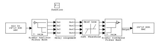
**Compatibility Considerations.** The V3.0 changes in the real-time scheduler can break some existing multirate models that contain codec blocks such as the ADC and DAC. The models affected contain at least one sample rate that is faster than the codec block rate. You do not run into this problem if all rates in the model are lower than the codec rate.
