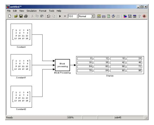
The Block Processing block operates on the submatrices, assembles the results into an output matrix, and then uses the Display block to present the output matrix. Dialog Box
