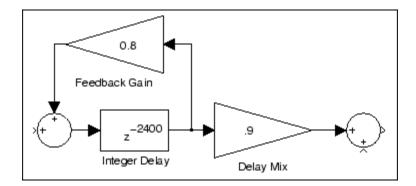
Look for the Integer Delay block in the Signal Operations library of the Signal Processing Blockset software. You do not need to add the input and output signal lines at this time. When you add the C6713 DSK blocks in the next section, you add the input and output to the sum blocks.
