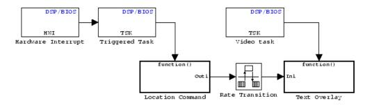
The DSP/BIOS Hardware Interrupt block installs an ISR function that signals a DSP/BIOS task to run when the ISR detects an RTDX<sup>™</sup> interrupt. Signaling between the ISR and DSP/BIOS triggered task occurs via semaphores. This task receives an RTDX message carrying the location command for the downstream Text Insert block in the Text Overlay from the host computer.
