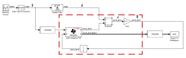
The portion of the model enclosed by the dashed line produces the signal B and feeds it back into the LMS Adaptive FIR block. The inputs to this region are  $\overline{X}$  and the desired signal d, and the output of this
